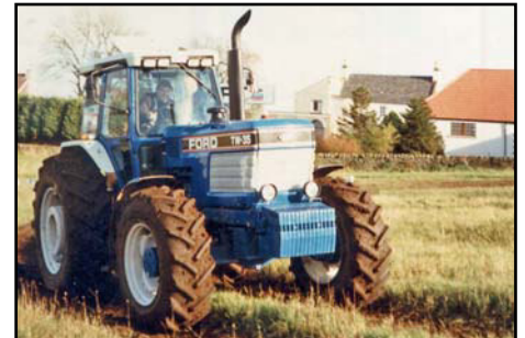
+ Ford TW35 AWD: 6.6-litre 6-cylinder turbo diesel, 192 bhp, 700 N.m torque, partial power-shift transmission, 16 forward gears, 4 reverse
