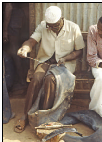
Darning punctures before sticking on the patches
